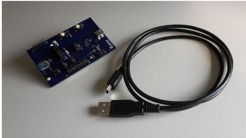
Figure 3: USB cable and evaluation board of the Proteus-I and Proteus-II radio module
